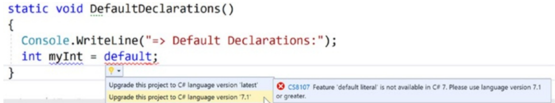
Figure 3-2. Upgrading the project to C# 7.1
